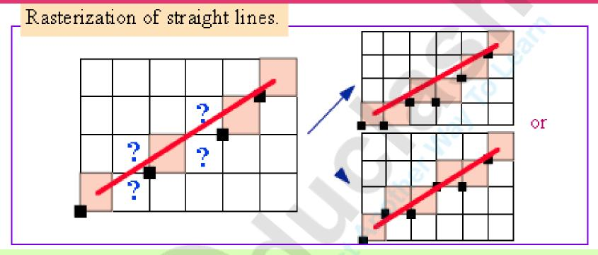
Rasterization yields uneven brightness: Horizontal and vertical lines appear brighter than the 45° lines.
