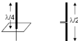
Fig: Shape of antenna proportional to wavelength
