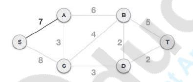
Now, the tree S-7-A is treated as one node and we check for all edges going out from it. We select the one which has the lowest cost and include it in the tree.
