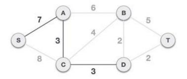
After adding node  $\mathbf{D}$  to the spanning tree, we now have two edges going out of it having the same cost, i.e. D-2-T and D-2-B. Thus, we can add either one. But the next step will again yield edge 2 as the least cost. Hence, we are showing a spanning tree with both edges included.
