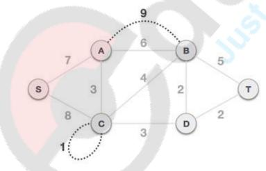
Remove all loops and parallel edges from the given graph. In case of parallel edges, keep the one which has the least cost associated and remove all others.
