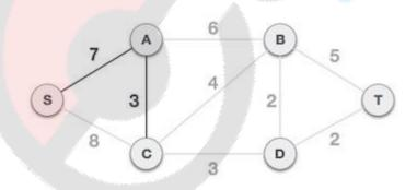
After this step, S-7-A-3-C tree is formed. Now we'll again treat it as a node and will check all the edges again. However, we will choose only the least cost edge. In this case, C-3-D is the new edge, which is less than other edges' cost 8, 6, 4, etc.
