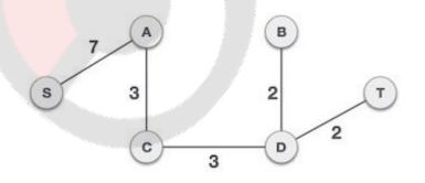
By adding edge S,A we have included all the nodes of the graph and we now have minimum cost spanning tree.
