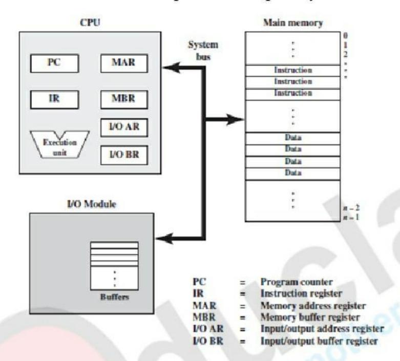
Central processing unit (CPU): Controls the operation of the computer and performs its data processing. That contain following unit-
