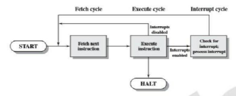
Instruction cycle with Interrupt referred to as the Fetch Cycle and Execute Cycle and interrupt cycle.
