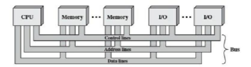
Any bus line can be classified into three functional groups that are DATA, ADDRESS and CONTROL
