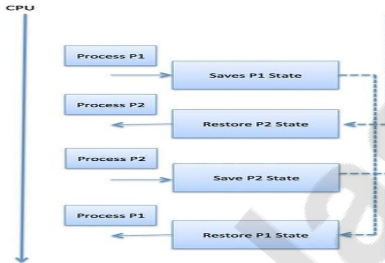
Context switches are computationally intensive since register and memory state must be saved and restored. To avoid the amount of context switching time, some hardware systems employ two or more sets of processor registers. When the process is switched, the following information is stored for later use.
